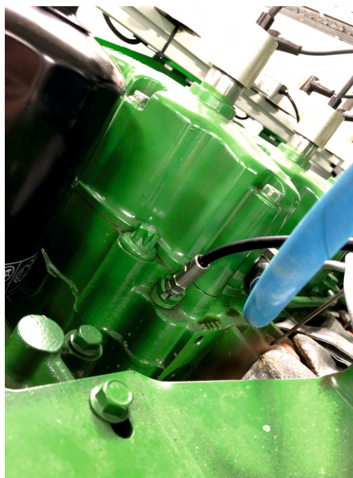
CPS-03 installed on a hydrogen engine
