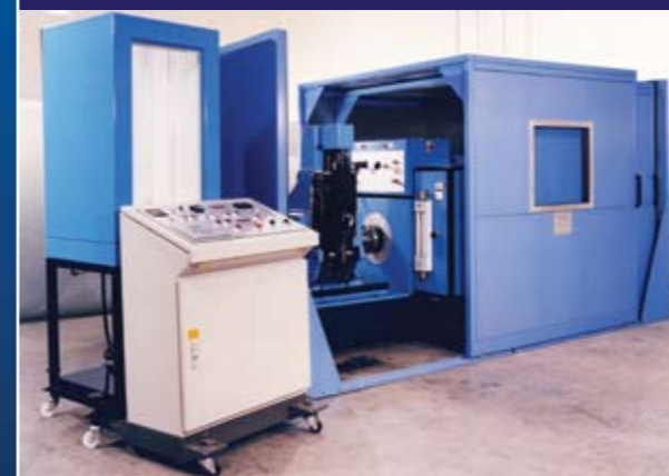
MK6 HD TEST STAND IN SOUNDPROOF ENCLOSURE WITH MOBILE CALIBRATION RIG & REMOTE CONTROL UNIT
