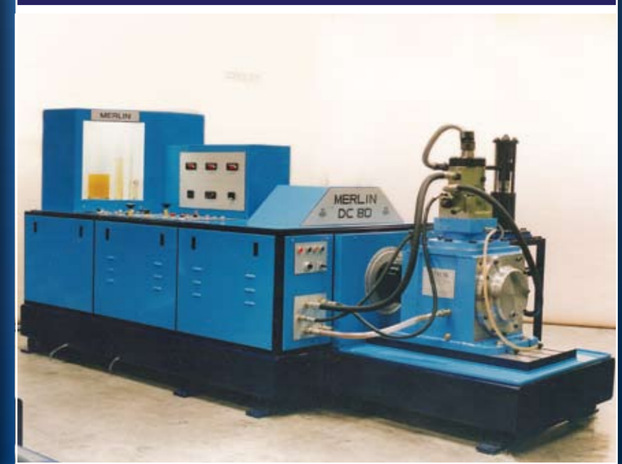
MERLIN DC80 HD TEST STAND AND MPC300-1 UP-RATED CAMBOX WITH SULZER ZA40S FUEL PUMP ON TEST
