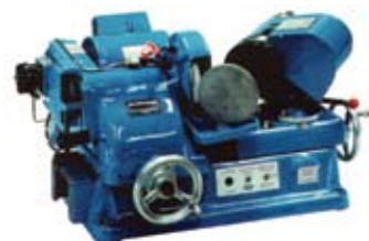
VM1 4" CHUCKS...1" (25MM) CAPACITY VM5 5" CHUCKS...1.5" (38MM) CAPACITY
