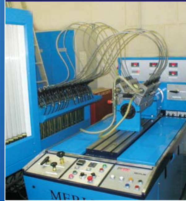
MERLIN H1230E TEST STAND WITH PA4-200 PUMP ON TEST...IDEAL FOR RAIL & MARINE APPLICATIONS
