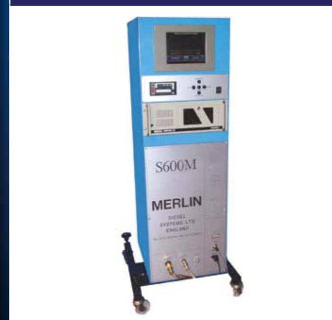
MERLIN S600M/5 METERING UNIT ...CAN BE FITTED TO ANY HD TEST STAND
