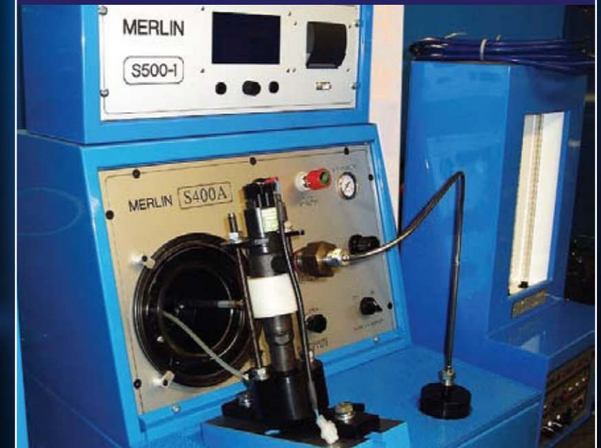
MERLIN S400A-CR PNEUMATIC INJECTOR TESTER WITH A MARINE COMMON RAIL INJECTOR ON TEST
